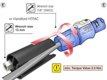
(SW 22) or with the Neutrik handtool HTFAC, min. Torque 2.5 Nm (1.8 lb-ft).
