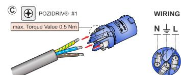
© Insert the wire into the terminals and fasten the clamping device with a POZIDRIV® #1, max. Torque 0.5 Nm (0.37 lb-ft).
